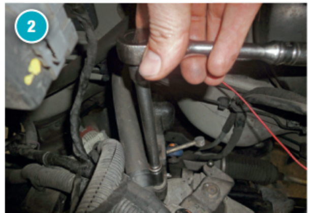
Next remove the 13mm counterweight bolt and counterweight. Please note that these are opposite sides on the GT and VTS!
