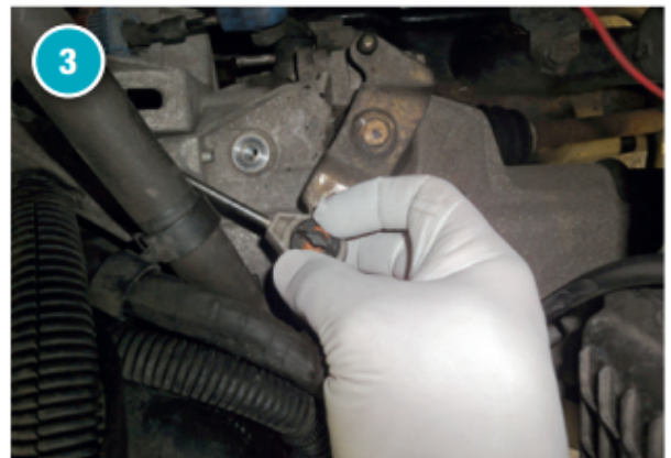
Remove the linkage cables by pressing the little orange tabs inwards, before pulling the cable end upwards. Be careful as they are fragile and it is a little fiddly. You need to remove both linkage cables in the same way.
