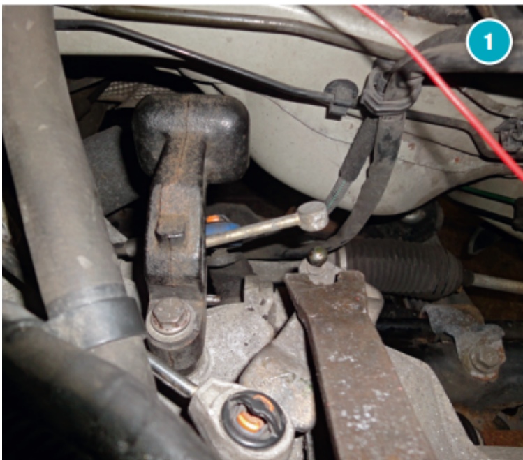
First off you need to remove the airbox, or filter, whichever you have, to allow access to where we need to be. Then you need to remove the linkage rod which connects the counter balance weight to the selector. You can do this easily by using a pry bar under one end of the linkage.
